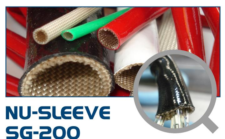
NU-SLEEVE SG-200 is a braided fiberglass sleeve coated with a liquid silicone rubber. The braid is heat treated to optimize coating adhesion and minimize surface irregularities.
